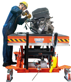
CMM Trolley with lift table for engine handling and dismantling.
